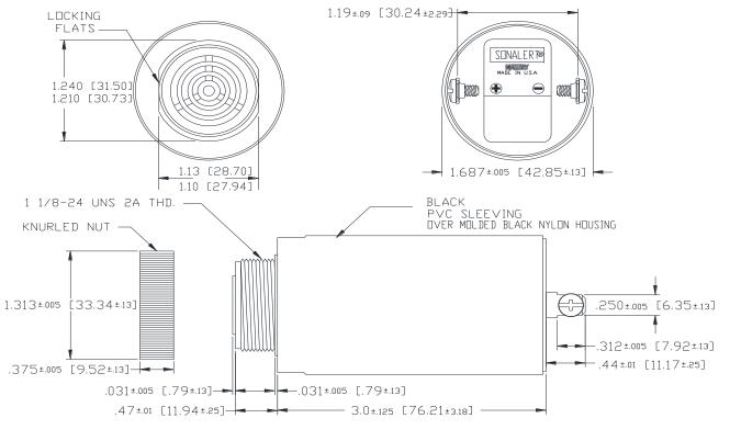
NOTE A: TERMINALS-.032 BRASS TIN PLATED, TAPPED FOR #6-32 SCREW. TWO #6-32 NICKEL PLATED BRASS SCREWS INCLUDED. WILL ACCEPT 1/4" QUICK CONNECT. NOTE B: MOUNTING- REMOVE BLACK PLASTIC NUT AND INSERT THREADED FRONT THROUGH 1.25" HOLE PUNCHED IN PANEL, IF ORIENTATION IS NEEDED, NOTE LOCKING FLATS ON DRAWING. SCREW NUT BACK ON. DO NOT OVERTIGHTEN.
